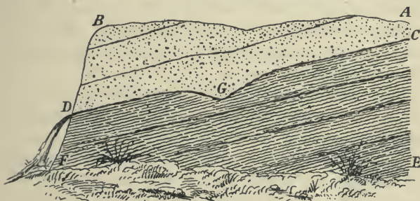
FIG. 6.—Formation of a spring.
